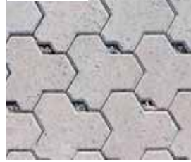
PERMEABLE UNIT PAVERS (P4a) 88mm x 181mm x 80mm Type: 'Ecotrihex' paver with gravel infill Colour: Oatmeal Supplier: Adbri Masonry
