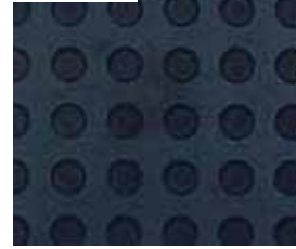
TACTILE INDICATORS 300mm x 300mm x 40mm Type: Pre-cast concrete paver Colour: Black Supplier: Chelmstone or equivalent
